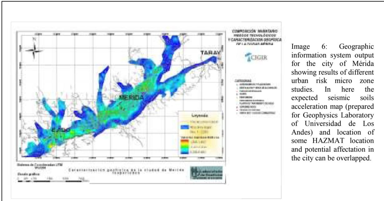
Image 6: Geographic information system output for the city of Mérida showing results of different urban risk micro zone studies. In here the expected seismic soils acceleration map (prepared for Geophysics Laboratory of Universidad de Los Andes) and location of some HAZMAT location and potential affectation in the city can be overlapped.
